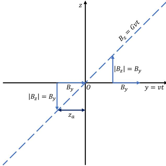
**Fig. S2.** Illustration of the magnetic field versus the y location of the atom in the inner rotation chamber (i.e., the middle stage). y denotes the axis of the atomic beam. Here,  $B_y > 0$ , and  $G = \partial B_z / \partial y > 0$ . For a given current,  $B_y$  is invariant with y while  $B_z$  is proportional to y (i.e., negative for  $y < 0$ , zero at  $y = 0$ , and positive for  $y > 0$ ). At  $y = \pm z_a$ , we have  $B_z = \pm B_y$  or  $|B_z| = B_y$ .
